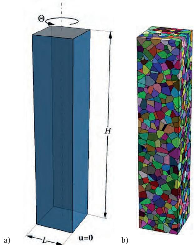
Fig. 7: Torsion test of a square-section bar. a) Geometry and boundary conditions and b) Voronoi mesh.
